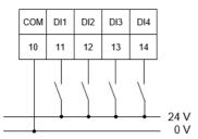
Power supply: 24 V AC/DC, connection via terminals
