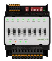
The digital output module romod 8 DO-R is a Local Override/Indication Device (LO/ID) which is used to control eight 1-stage motors, or other digital actuators. By means of the integrated switches, it provides the ability of manual override of the DOs which are usually controlled via Modbus commands.
