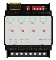
The digital output module romod 4 DO-R is a Local Override/Indication Device (LO/ID) which is used to control four lighting circuits, or other digital actuators. By means of the integrated push buttons, it provides the ability of manual override of the DOs which are usually controlled via Modbus commands. The relay outputs provide the normally open contact of each relay and will be contacted via terminals. They are implemented using bistable relays.
