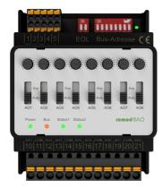
The analog output module romod 8 AO is a Local Override/Indication Device (LO/ID) which is used to provide eight 0-10V control signals. These may be utilized, e.g., for controlling heating valves, dampers or frequency converters etc. By means of the integrated switches and potentiometers, it provides the ability of manual override of the AOs which are
