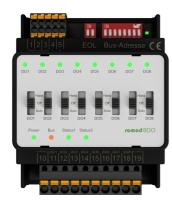
The digital output module romod 8 DO is a Local Override/Indication Device (LO/ID) which is used to control eight 1-stage motors, or other digital actuators. By means of the integrated switches, it provides the ability of manual override of the DOs which are usually controlled via Modbus commands.
