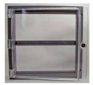
The mounting frame RTR7050S is used for the installation of 12 romutec control modules with 8 TE width. You can mount various 19" modules, i.e. up to 12 romutec modules (width 8TE and height 3HE). The modules will be mounted with screws M2,5. The mounting frame will be attached to the cabinet's door with 4 screws M6 (Type FKSM6, included in delivery). The frame covers the cutting edges. The dimensions are shown in the drawing.
