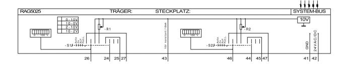
Power supply: 24V AC/DC, ±10% Consumption max. 80 mA
