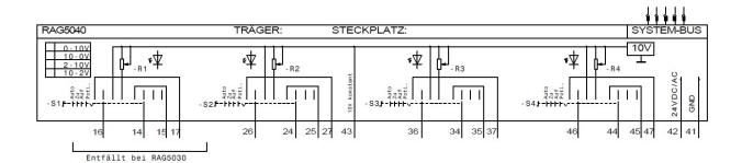
Power supply: 24V AC/DC, ±10% Consumption max. 80 mA
