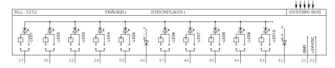
Power supply 24V DC, ±10% Current consumption max. 120 mA (per LED about 5 mA)
