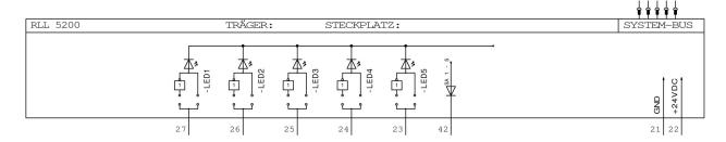
Power supply 24V DC, ±10% Current consumption max. 120 mA (per LED about 5 mA)
