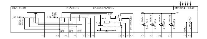
Supply voltage: 24V DC / AC ± 10% Power consumption: max. 110 MAPRO relay 15 mA) (Per LED about 5 mA)
