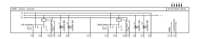
Supply voltage: 24V DC / AC  $\pm$  10% Power consumption: max. 110 MAPRO relay 15 mA) (Per LED about 5 mA)
