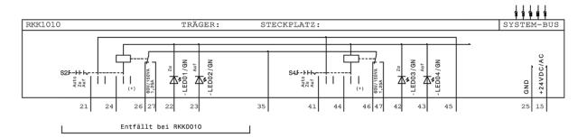
Supply voltage: 24V DC / AC ± 10% Power consumption: max. 110 MAPRO relay 15 mA)
