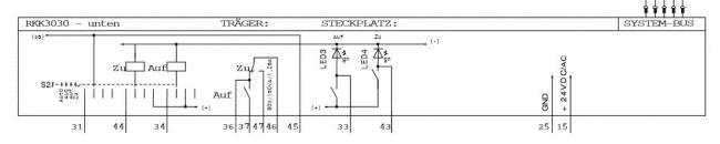
Supply voltage: 24V DC / AC ± 10% Power consumption: max. 110 MAPRO relay 15 mA) (Per LED about 5 mA)
